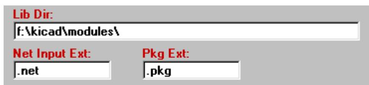
**Lib Dir** is the default path of the footprint file (**.mod**) and of the equivalence (**.equ**) files. If this field is left empty, the default path used will be **kicad/modules**.
