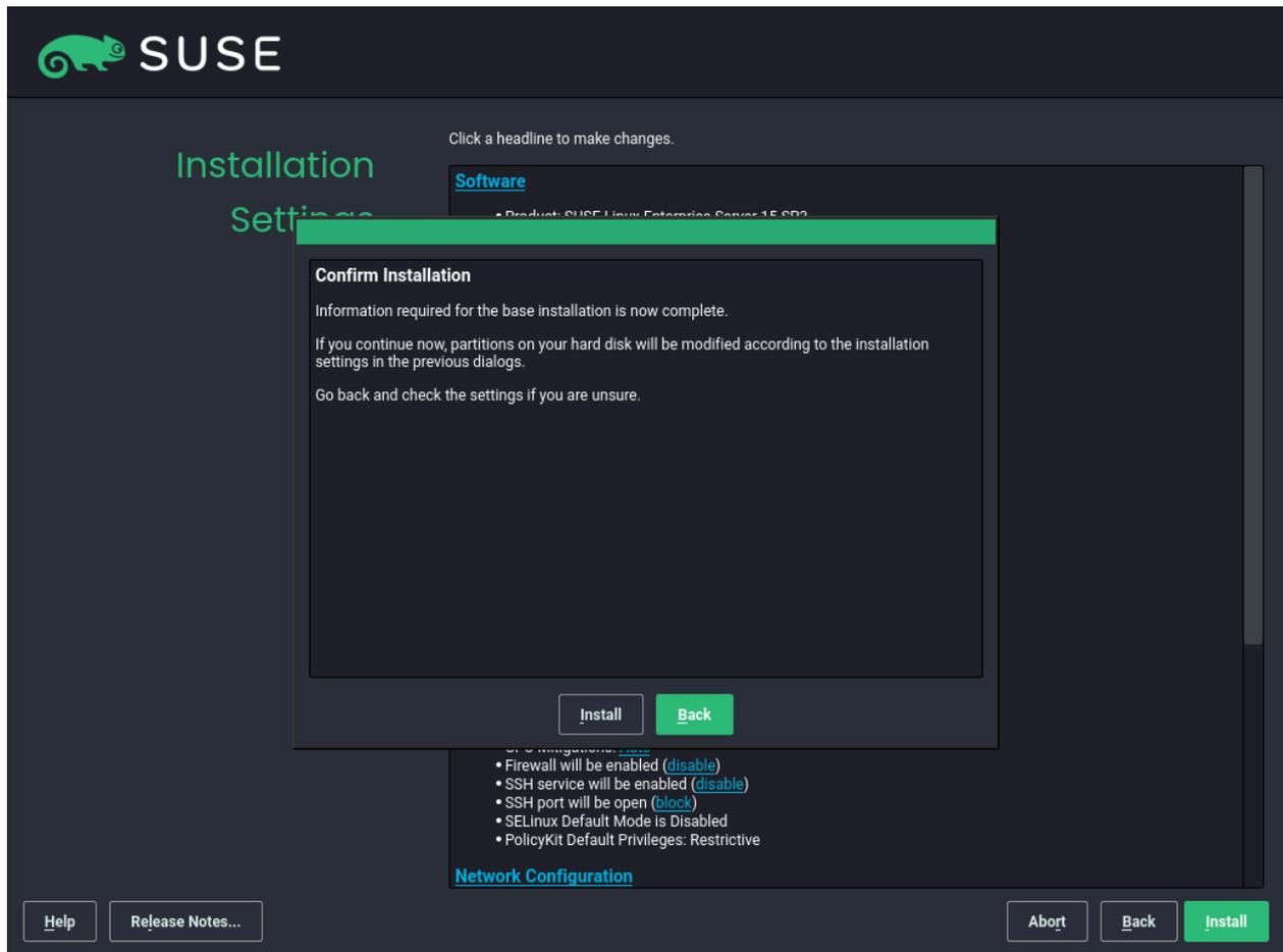
After you have finalized the system configuration on the *Installation Settings* screen, click *Install*. Depending on your software selection you may need to agree to license agreements before the installation confirmation screen pops up. Up to this point no changes have been made to your system. After you click *Install* a second time, the installation process starts.
