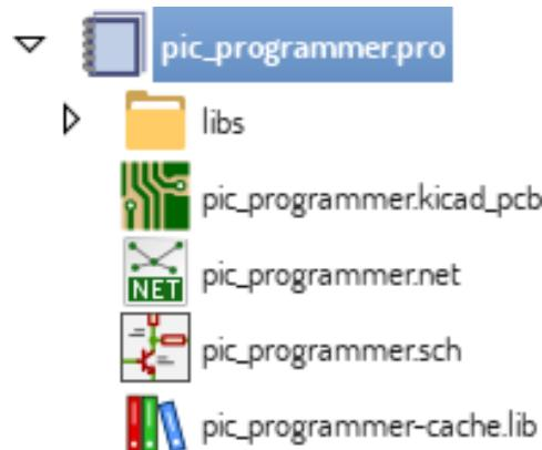
Double-clicking on the schematic file runs the schematic editor, in this case opening the file **pic\_programmer.sch**.
