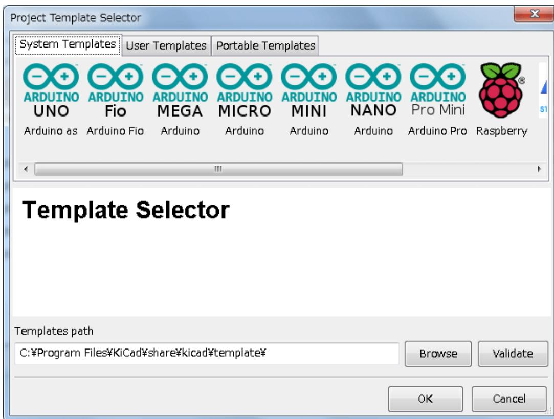
A single click on a template's icon will display the template information, and a further click on the OK button creates the new project. The template files will be copied to the new project location and renamed to reflect the new project's name.
