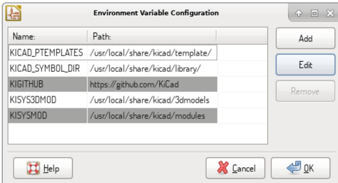
Note also the environment variable **KIPRJMOD** is **always** internally defined by KiCad, and is the **current project absolute path**.
