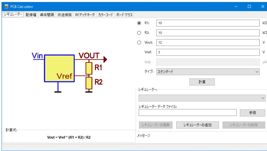
For the *Standard Type*, the output voltage  $V_{out}$  as a function of the reference voltage  $V_{ref}$  and resistors  $R_1$  and  $R_2$  is given by:
